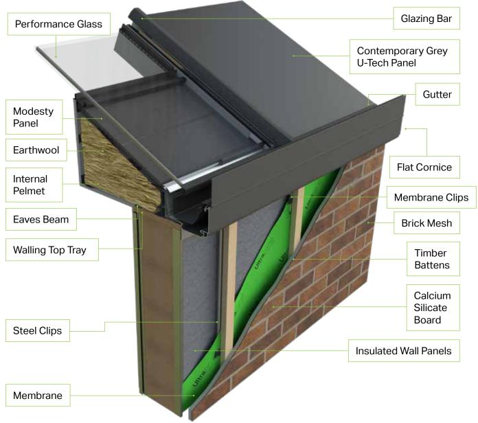
The hup! Hybrid Roof is available for roof pitches from 5° to 40° is fully configurable to any shape and size. Combining unique contemporary grey panels with rectangular or shaped glazed panels. The hup! Hybrid Roof is based on Livinroof by Ultraframe.
