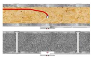
Drill hole through top tray and EPS to thread conduit through.
