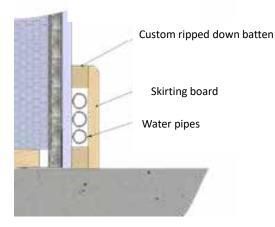
Skirting boards can be purchase with a ready made void for pipes as shown to the right.
