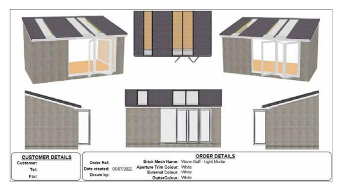
This shows a 3D representation of the hup! from all sides. A single glazed roof panel lights the utility room, and bi-fold doors and a double glass roof panel provide plenty of natural light into the lounge. Both boundary walls are solid with no windows. White gutters and roof trims have been chosen and the walls are shown with the hup! Brick Mesh in Warm Buff with Light Mortar.
