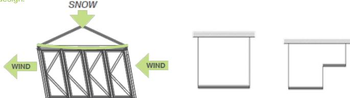
Downward, vertical forces (e.g. snow) need to be managed to prevent doors from sticking and lateral forces from side winds need to be managed to prevent the building from racking.
