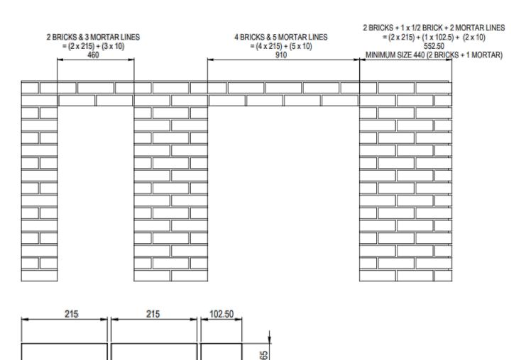
STANDARD UK BRICK SIZES LAYOUT BASED ON BRICK & HALF BRICK
