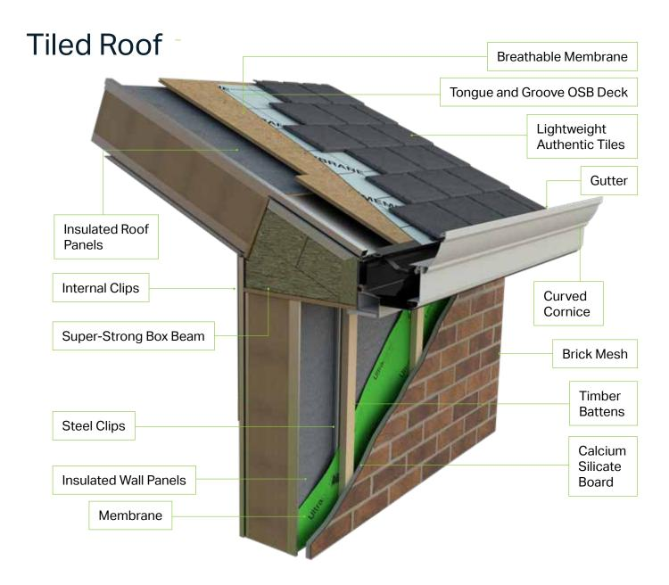
The hup! Tiled Roof is also known as Ultraroof and does not need a tie bar like other lightweight Tiled Roof systems (although for gable and lean-to roofs a high level strut may be needed, see page 35). Available with a choice of full length glazing panels in a range of high performance glass or conventional Velux windows, the roof can accommodate door spans of up to 4m with no need for extra structural support.
