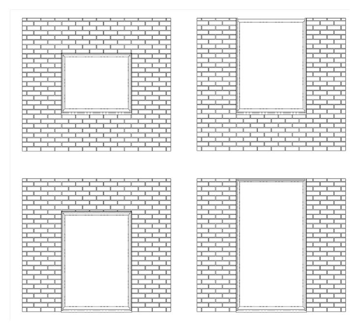
If using the hup! corner, apertures must be a minimum of 275mm from the corner of the base.
